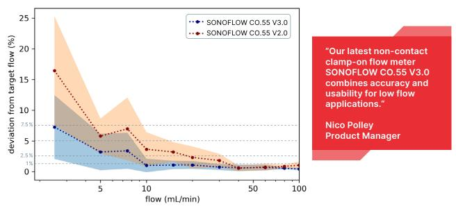
Plot: Testing of SONOFLOW CO.55 V3.0 and SONOFLOW CO.55 V2.0 in low flow measurement
