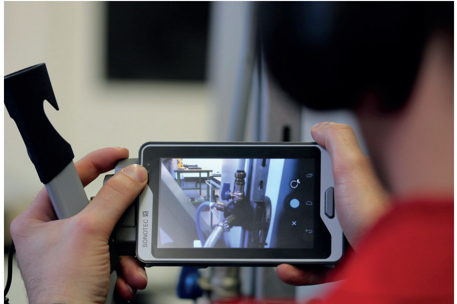
Images of the leak can be taken with the integrated camera
